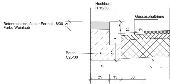
Detail zu C2: Pflaster/Hochbord/Gussasphaltrinne/Fahrbahn
